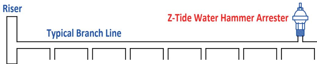
As shown, it has been established that the preferred location for the water hammer arrester is at the end of branch line between the two fixtures served.
