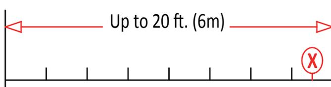
**Rule 2** covers multiple fixture branch lines which do exceed 20 ft. (6m) in length.
